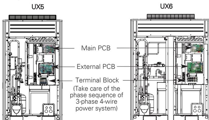
**Wiring of main power supply and equipment capacity**
