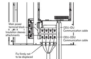
**Example) Installation of IO Module**
