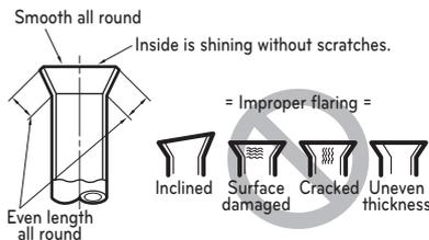
**Flare shape and flare nut tightening torque**
