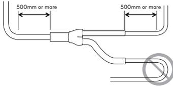
**Pipe Connection Method/Precautions for Series connections between Outdoor units**
